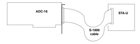
Figure 1. Connecting the ADC-16 Board to an STA-U
